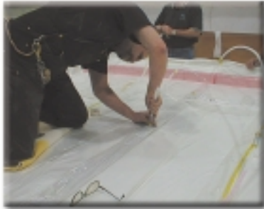
Above: Rick Schafer carefully installing resin supply line.
