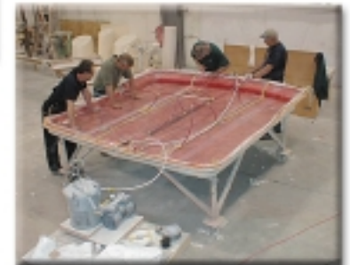
Right: Completed part - 22 minutes from start of infusion to completion.
